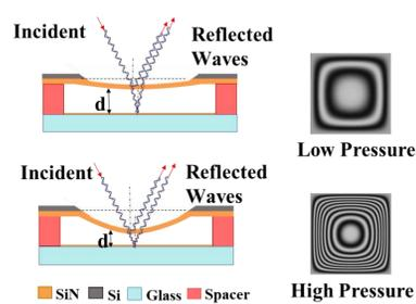
The sensor is designed based on the principle of interferometry. When monochromatic light is directed towards the sensor, reflected light waves from the bottom surface of the SiN diaphragm interfere with the reflected waves from the top surface of the SiN-coated glass substrate creating bright and dark fringes. The optical read-out of the sensor is captured using a camera and post-processed using image processing algorithm to correlate fringes pattern with pressure.
