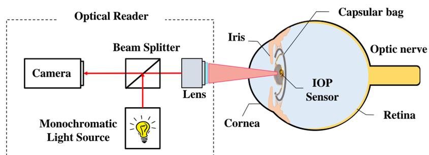
The measurement system consists of a hand-held reader designed to capture interferometric patterns from the implanted optical sensor. As shown in the figure above, the sensor is integrated onto an intraocular lens and implanted during standard cataract surgery. By directing the monochromatic light emitted from the reader towards the sensor, one can obtain the interference pattern and, consequently, the intraocular pressure.
