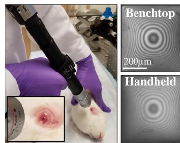
To demonstrate the feasibility of the system for point-of-care applications, the benchtop microscope set-up was replaced with a portable hand-held reader. The hand-held reader with a CMOS camera attachment can be directed towards the sensor implanted in the rabbit eye. The same fringe pattern can be observed in both the benchtop and the hand-held device, indicating the successful use of a portable readout system.
